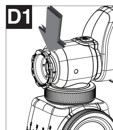
**⚠ CAUTION:** Do not compress or push spring when adjusting fan pattern. The nozzle should rotate and not loosen.
